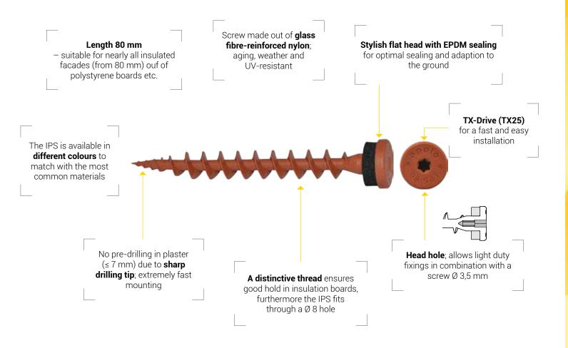
Insulation screw IPS is perfectly suitable for direct fastening into insulation materials without thermal bridges of wall connection profiles, metal sheets, base protection profiles, cornice covers, motion detectors, lamps, signs, etc.
